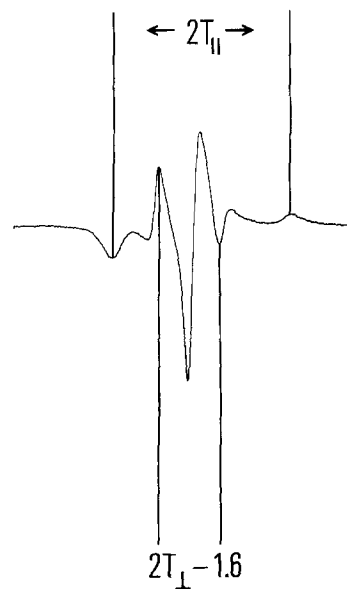
Fig. 1. A typical electron spin resonance spectrum of spin labeled renal brush border membranes. From such spectra, the hyperfine splittings T_{\parallel} and T_{\perp} were calculated as described in the text
